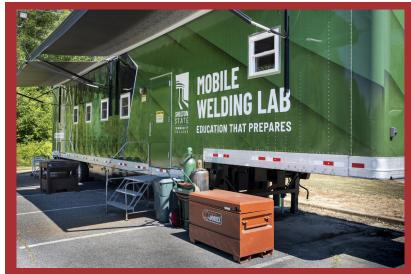
trailer has an on board Fike fire suppression system and two fire extinguishers. A Hypertherm Powermax 45 xp plasma cutter is utilized for outside cutting and gouging.
